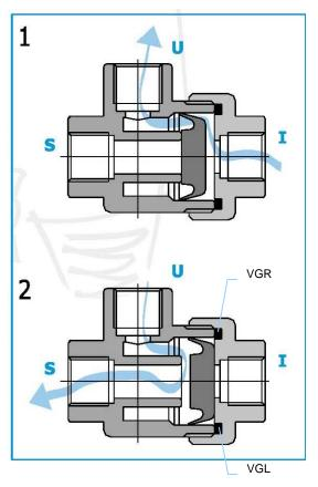
THE AIR ENTER IN THE "I" ENTRY AND, MOVING THE SEAL PACKING, IT PASSES AT THE USE "U" DIRECTLY.
